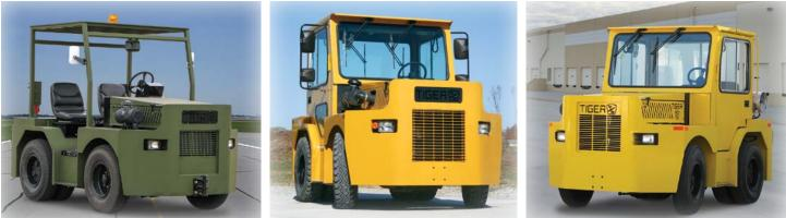
The TC-80/120 heavy duty tow tractor is a proven product with 8,000-12,000 pounds (36-54 kN) of drawbar pull.
