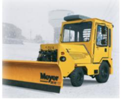
The TC-30/60 tow tractor is designed to provide a versatile and highly maneuverable solution for your towing requirements demanding 3,000-6,000 lb (14-27 kN) of drawbar pull.
